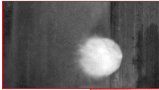
Left: Photo 2. Ice Sphere at Moment of Impact with Concrete Tile.
